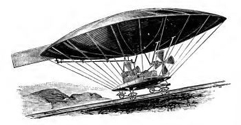
The vertical direction of the balloon is regulated by an adjustable weight, or by increasing or decreasing the speed of the propellers.
